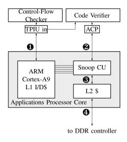
Fig. 1. High level overview of LAHEL. Our IP core interfaces with the TPIU, **0**, to extract control-flow information. TPIU traces are decoded and forwarded to the control-flow checker and code verifier. Program code is read through an AMBA AXI master connected to the Snoop Control Unit, **0**, which reads code from the L2 cache **6**, forwarding any misses to the DDR controller, **6**.
