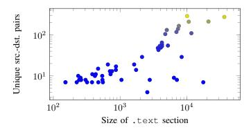
Fig. 3. Distribution of unique indirect control-flow transfer address pairs in the BEEBS benchmark suite compiled for the ARMv7-A architecture. We only include the integer subset of the benchmarks in our analysis. Root of trust routines are not included in this plot.
