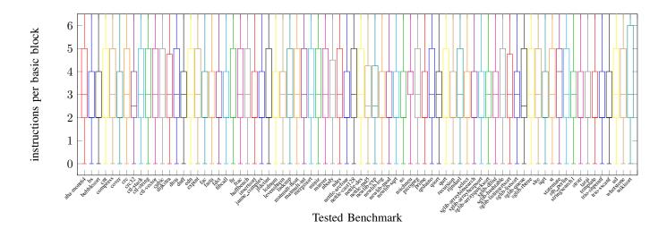
Fig. 4. Average instruction count per basic block in BEEBS. We exclude outliers in our plots, which we define to be 2.5 standard deviations away from the mean value of instructions per basic block for a particular benchmark. Benchmarks exhibit an average of three instructions per basic block. This implies that under the ARM ISA a basic block is 12 B (96 bit) in size.
