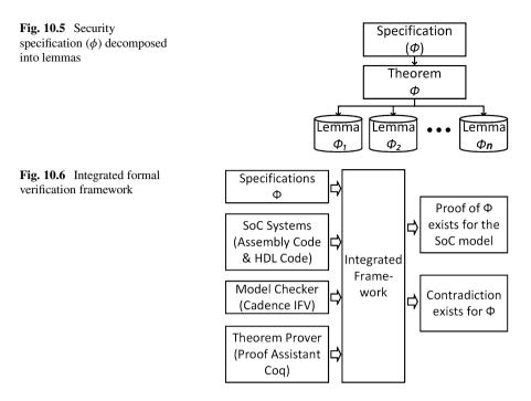
the security properties are checked against SoC designs. In this framework, the theorem prover is combined with a model checker for proving formal security properties (specifications). Moreover, the hierarchical structure of the SoC is leveraged to reduce the verification effort.
