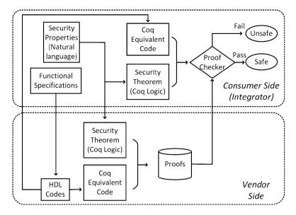
Fig. 10.3 Working process of the PCH framework [17]
