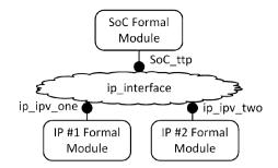
modules such as IP #1 Formal Module or IP #2 Formal Module in the figure. The *ip\_ipv\_one*, *ip\_ipv\_two*, and *SoC\_ttp* are the name of the corresponding *interfaces*.
