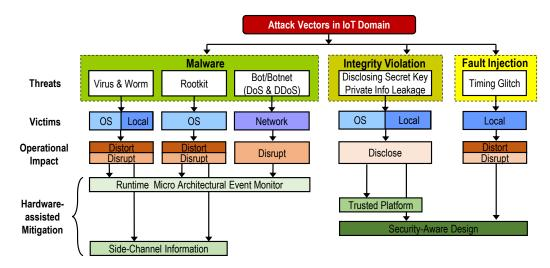
Fig. 1. Common cyber-attacks for IoT devices and hardware-assisted mitigation techniques.
