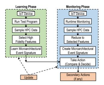
Fig. 2. Hardware Performance Counter-based Malware Detection.
