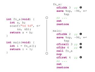
Fig. 1. HAFIX++ instrumentation. The compiler inserts new instructions before and after call/jump instructions, as well as in function entries and targets for indirect jumps.
