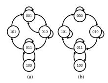
Fig. 2: The two FSMs recovered from the RS232 netlist. (a) First decomposed FSM and (b) second decomposed FSM.
