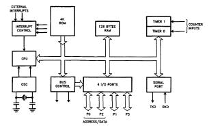
Fig. 4. Block Diagram of the 8051 Microprocessor [10]
