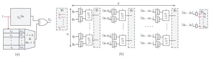
Fig. 3: (a) EFS-security can be guaranteed by flipping the output of  $c_o$  on p input patterns and correcting it using a conditional-look-up function implemented with TCAM logic with  $z \ge p$  entries. (b) Universal circuit with depth d and width w. The blue wires are key-variables, and the red wires are input-outputs.
