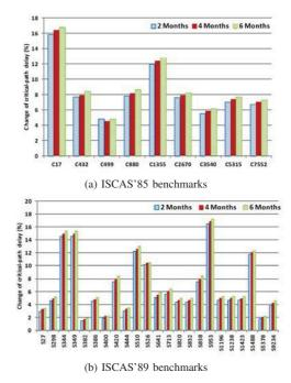
Fig. 5: Percentage change in critical-path delay of benchmark circuits as a function of attack duration.
